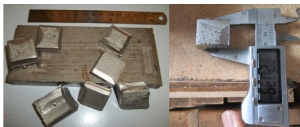
Figure 1. Pure nickel as basic material of BNCT collimator
