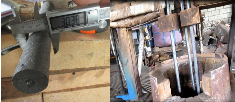
Figure 2. Graphite Electrodes and Electric Arc Furnace with 3 graphite electrodes
