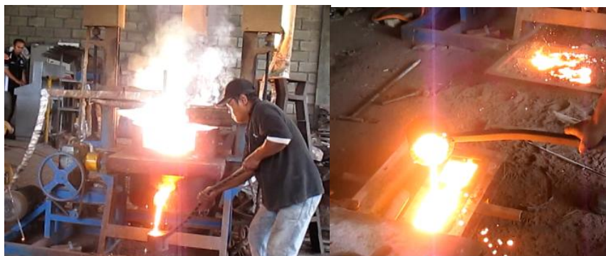
Figure 5. The discharge process of nickel from the furnace chamber and pouring it into the molding
